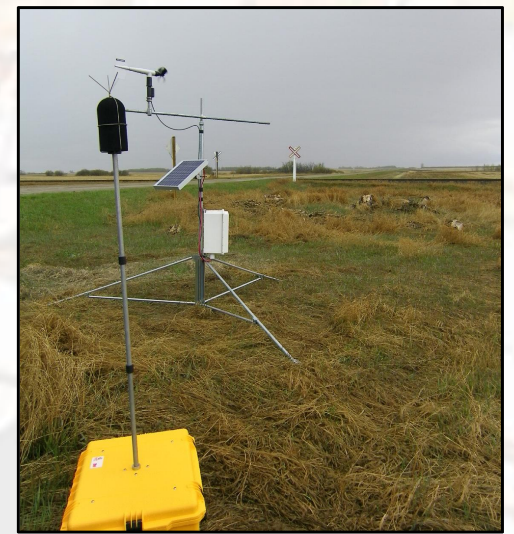
Noise monitoring equipment including microphone, anemometer, data logger and solar panel
